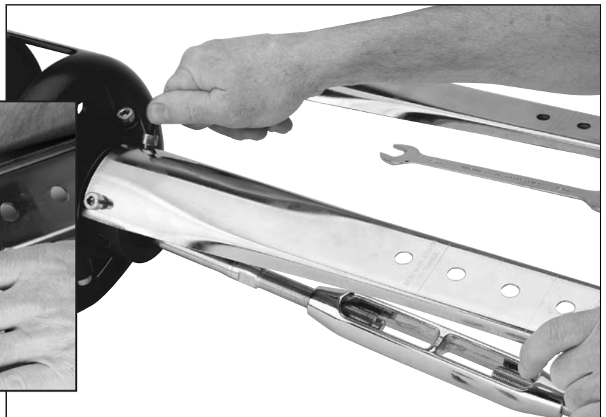
Toggle For Long Link Plates
