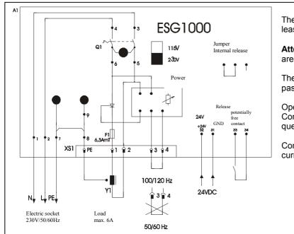
The jumper must be diverted to enable the external release.
