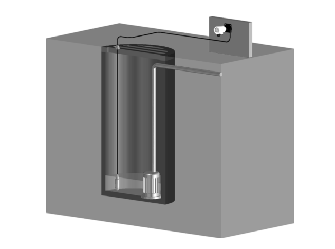
Fig. 5: Mounting example: Version with suspension cable in a pump shaft
