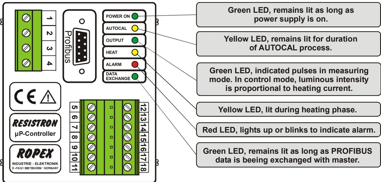
In addition to the functions shown in the diagram above, various controller operating states are indicated
