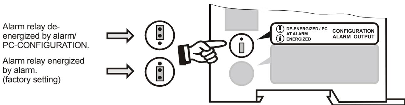
**!** If the jumper is not inserted, the alarm relay is permanently energized. The other functions of the controller (e.g. heating, AUTOCAL etc.) are not impaired by this.
