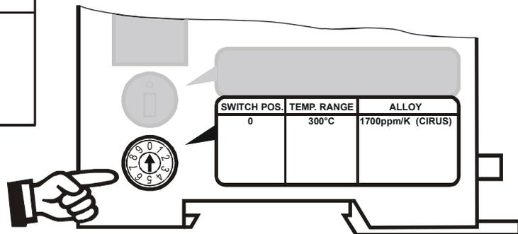
**!** The setting of the rotary coding switch for the temperature range and alloy can be overwritten with the parameter data (↪ section 9.6 "Parameter data" on page 24).
