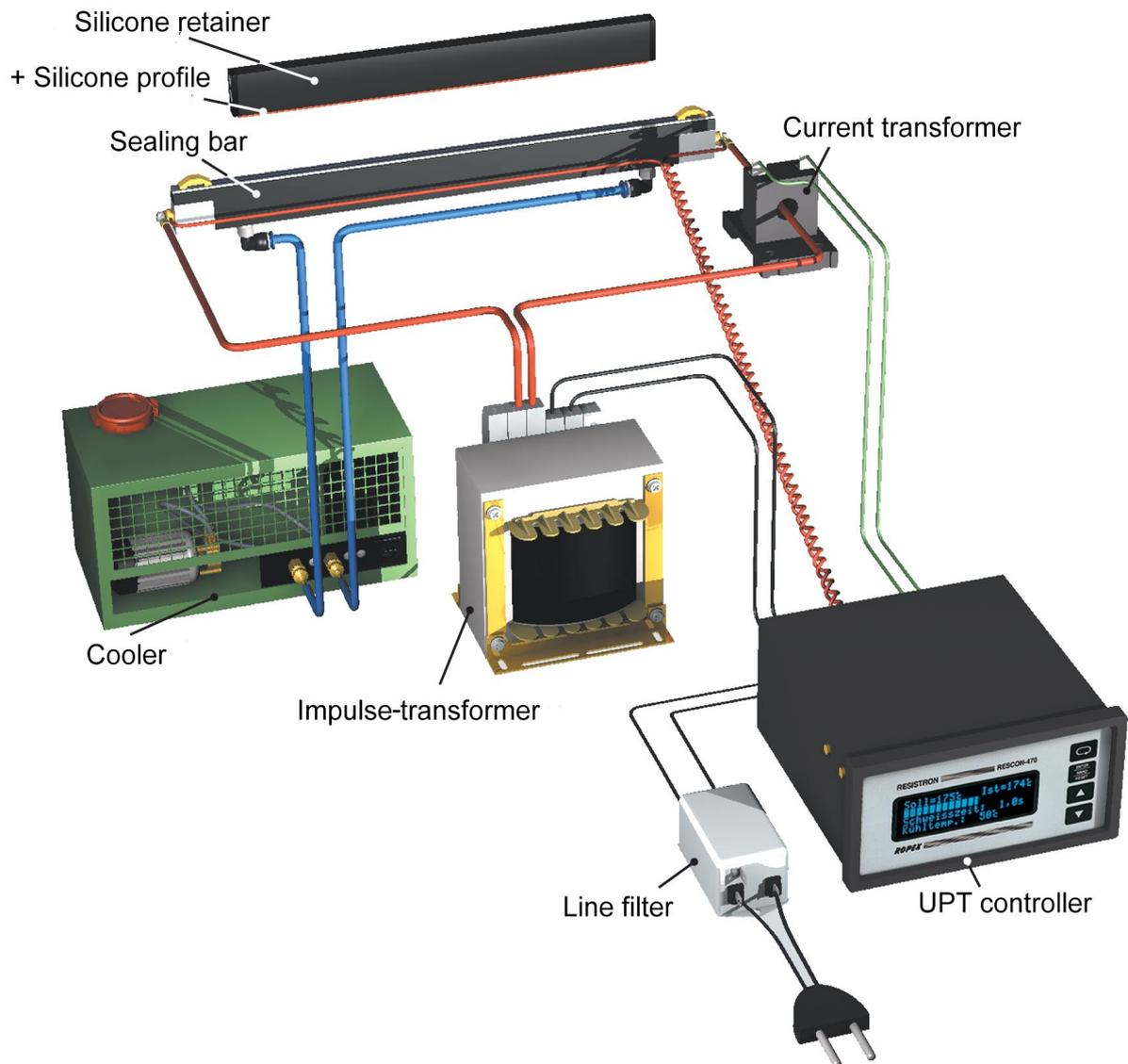
The basic design of the overall system is shown in the diagram above.
