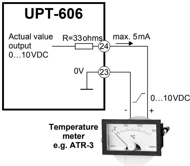
The characteristics of the ROPEX ATR-3 temperature meter (size, scaling, dynamic response) are ideally suited to this application and this instrument should therefore always be used (↪ section 4 "Accessories and modifications" on page 6).
