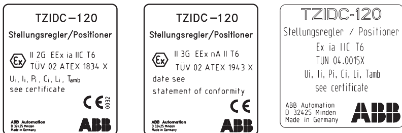
Fig. 1 Type plate indicating the degree of explosion protection
