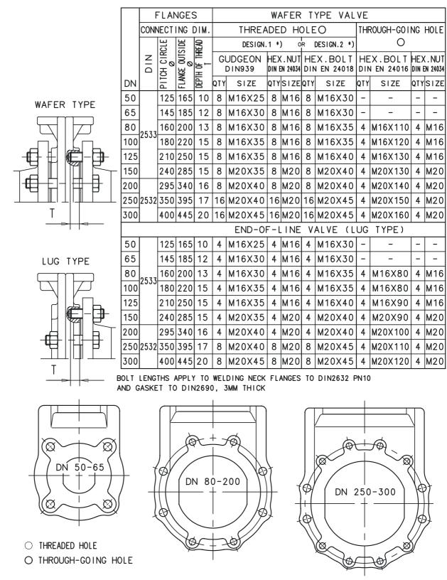
\*) FOR FASTENING THE GATE VALVE TO THE PIPELINE, WE RECOMMEND DESIGN 1 (GUDGEON AND NUT) FOR THREADED HOLES, AS THIS DESIGN USES THE WHOLE DEPTH OF THE THREAD.
