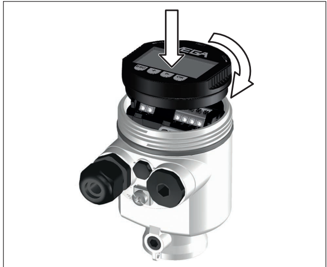
Fig. 29: Insertion of the display and adjustment module with single chamber housing
