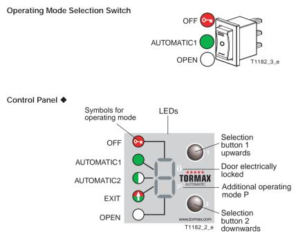
The control panel can display causes of malfunctions as well as the operating mode (see section 5)
