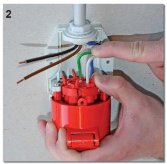
While pressing the release lever, bend one wire and insert into its terminal. Repeat this process until all wires have been placed in their designated terminal.
