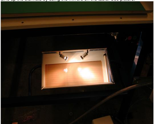
When you have the blanket in position and ready to cut, keep your hands on the blanket and in position, then press the pedal to do the cut.
