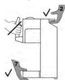
Hold the **Carrying handle** (2) and the **Instrument deck** (7) to lift VIAFLO 96.
