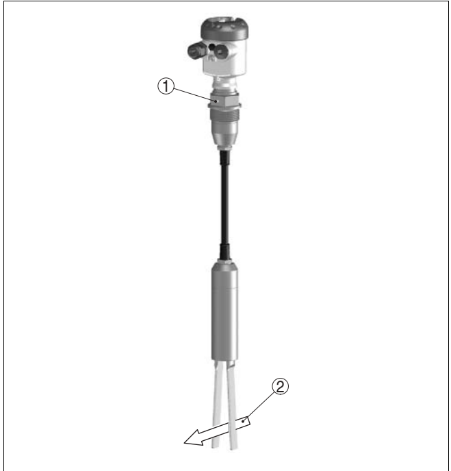
Fig. 6: Orientation of the tuning fork in case of flow 1 Marking with screwed version 2 Direction of flow
