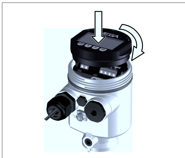
Fig. 6: Insertion of the indicating and adjustment module with single chamber housing into the electronics compartment
