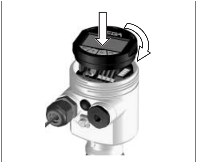
Fig. 18: Installation of the indicating and adjustment module
