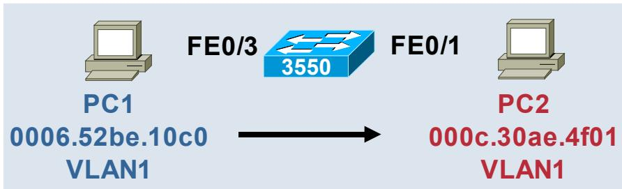
**How Would a Packet Sent from PC1 to PC2 Be L2 Switched in HW by the 3550?**
