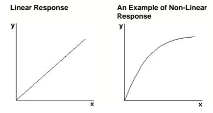
A linear response is one whose output-versus-input graph is a straight line. A typical example of this type of response is a photodiode.
