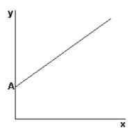
The above linear/non-linear responses could have a voltage/current/resistive, etc offset that may need taking into account. It is quite usual to see offsets in output signals from sensors.
