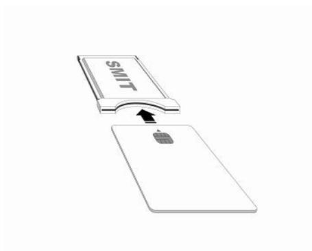
2. Insert the CAM into the IRD or monitoring equipment correctly. Please refer to the following figure. If the CAM is inserted properly, the TV screen will show CICAM initialization information.
