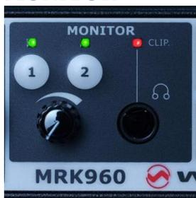
**Monitor 1** and **Monitor 2** activates monitor on jack output (6.3mm - 1/4") for receiver 1 and 2, respectively (a green LED is lighted when a receiver is selected). Audio level can be adjusted with the rotary knob. A blinking red led (CLIP) means clipping in the audio monitor output.
