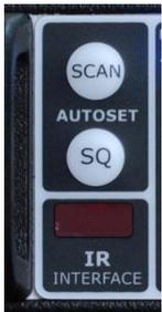
**SCAN** is an automatic scan function for all active frequencies of the selected group. This is a quick way to find the lowest noise frequency to work with.
