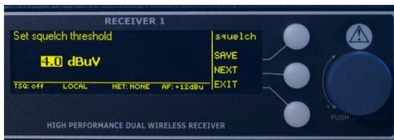
Rotate the knob to modify the squelch value in the allowed range (OFF to 1000  $\mu$ Volt or OFF to 60dB $\mu$ Volt, depending on the selected unit).
