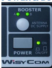
**BOOSTER** switch activates antenna powering (boosters) with 12VDC/200mA MAX for each antenna and the green LED is lighted (a blinking LED indicates a faulty condition; in this case power down the device and check for short circuits). Booster supply for antenna A and antenna B are independent, switchable from the *radio->options* menu.
