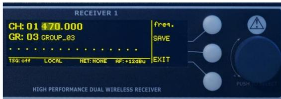
Current frequency can be quickly selected using the rotary knob. Push enter button or rotary knob to confirm current field editing and start modifying the following field (frequency integer part → decimal part, units=MHz).
