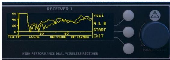
The WALK TEST menu allows a 90 sec recording of the received signal for A and B antennas; the result is displayed on the display. The sample rate is one sample per second but the value displayed in mode *A&B*, *A*, *B* (chosen with the first button) is the minimum level of the RF signal received on each antenna. Selecting *MAX AB* (pushing the first button), the maximum level of signal received is displayed.
