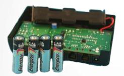
Insert 4 x AA rechargeable batteries in the battery pack..
