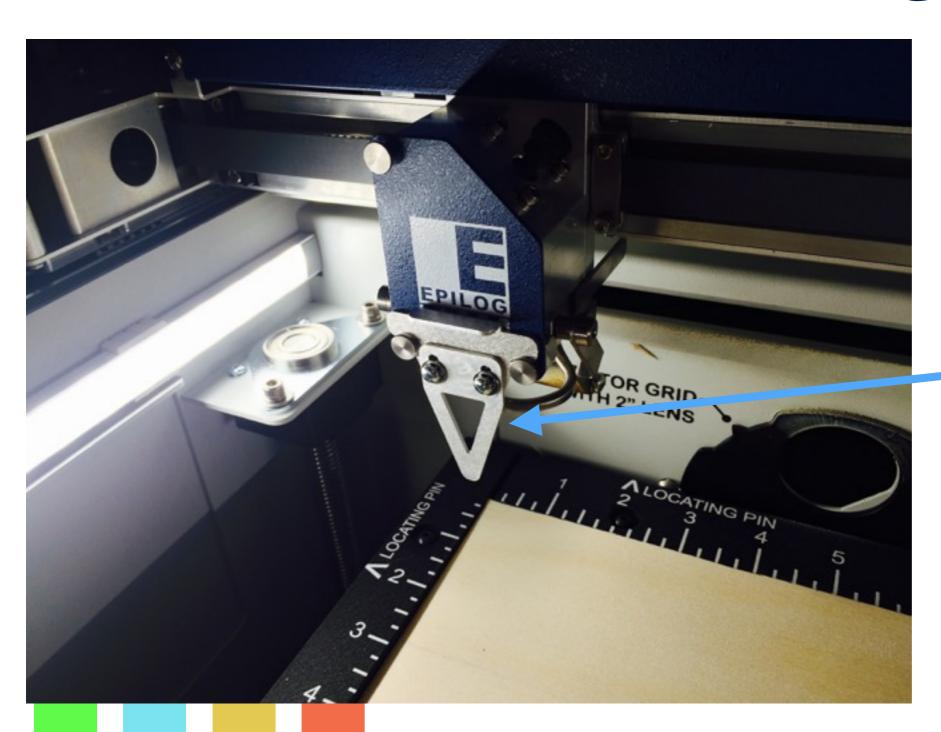
Put the height calibration piece on the cutter head.
