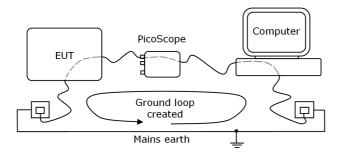
The majority of laptop power supplies (chargers) are floating and have no ground reference. If, however, connecting your grounded laptop power supply causes noise/offset problems, you can either use the oscilloscope with the laptop running on its batteries or power the oscilloscope using the supplied mains adaptor.
