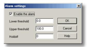
This dialog box defines the alarm settings for each measurement. It is invoked when you click the Alarm button on the **Parameter options** dialog box.
