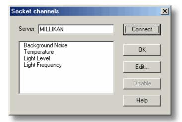
This dialog box is used to establish a connection to another instance of PicoLog running on a remote server computer, and then to select the channels that are to be imported to this instance of PicoLog.
