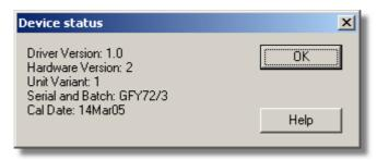
This dialog box displays the details about the HumidiProbe's status.
