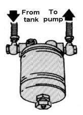
NOTE – the filter cartridge cannot be cleaned and used again.
