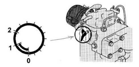
Turning the grip further – always clock-wise – will engage the automatic control. When the engine is cranked, the valve will automatically return notch by notch to the "0" position. This takes four full turns of the crank handle and the speed gained thereby should make the engine fire at the first following compression stroke.
