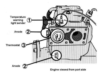
The self-sacrificing anodes – are checked regularly and replaced if more than 50% has been eaten away by corrosion. Undo the anodes – 2 – and replace them with new ones, including new gaskets.
