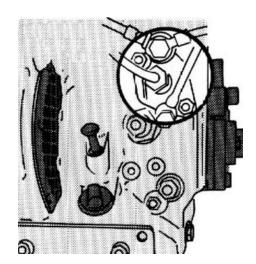
5. The injector – of Bosch manufacture, will normally need no maintenance except for cleaning of the area nect to the atomizer. The injector must not be dismantled, since the set injection pressure then could be altered inadvertedly.
