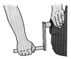
**Aloha Owners Association note** – owners of some Aloha 27s advise that due to the close proximity of the bulkhead there may be insufficient clearance to allow insertion of the crank handle for manual starting
