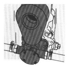
Pump impeller change – is possible when the pump housing front cover is removed. Pry the impeller off its shaft using two scredrivers. Lubricate the shaft and the impeller vanes with a few drops of oil prior to installation. Bend the vanes opposite to the direction of rotation in order to avoid distortion. Renew the pump housing gasket and install the cover.
