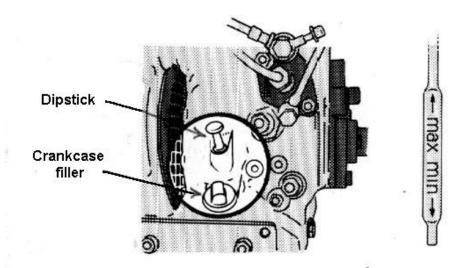
Engine oil change – normally every 50 hours. A brand new engine, however, will require it's first oil change after ten or fifteen hours running. Pump out the oil oil via the dipstick opening while the engine is warm. Refill via the crankcase filler plug.
