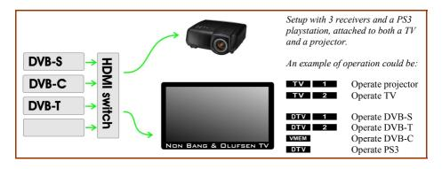
If the HDMI switch in the example is a beeLINK operated type, it will automatically switch to the last chosen source.
