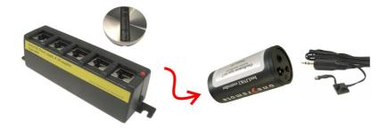
Data received by the IR-receiver is fed to a OneRemote Link Amplifier with built-in power supply and 5 outputs for beeLINK devices.
