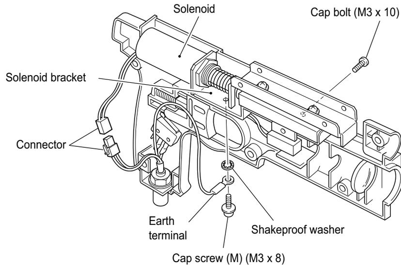
5. Loosen the nuts (16mm dia.) and remove the solenoid.
