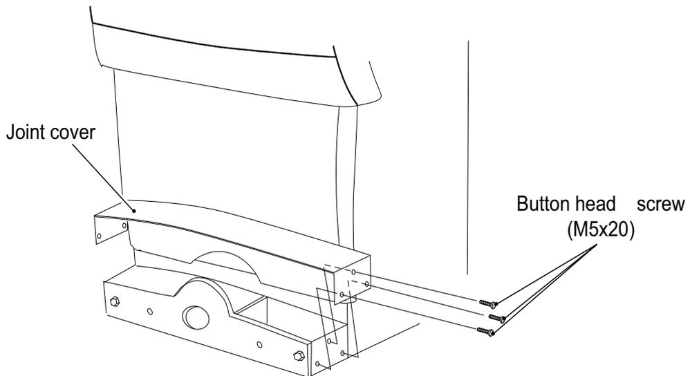
4. Place the Gun Cabinet close to the Monitor Cabinet and connect the connectors.
