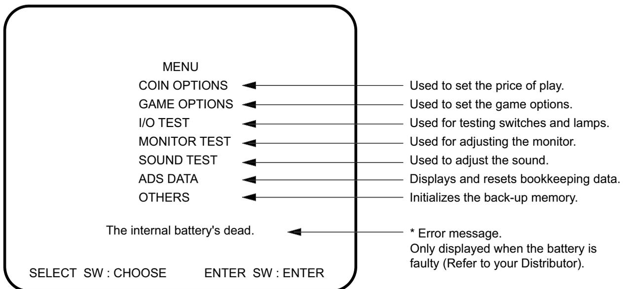
\* Error message (the internal battery is beginning to run down or is faulty.)
