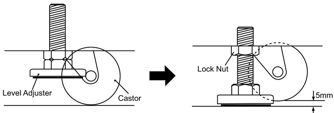
*Note: If the location site of this machine has a polished floor it is recommended that rubber pads are fitted under the level adjusters to prevent the machine sliding on the floor when in use.*
