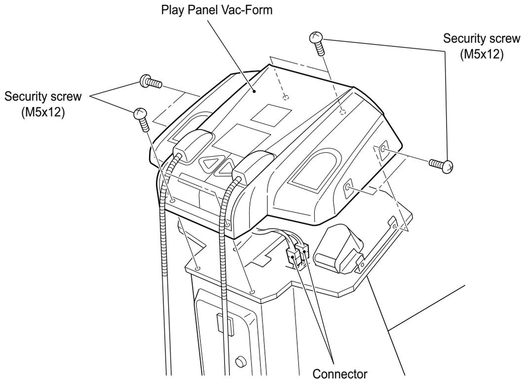
3. Disconnect the connectors and remove the Play Panel, complete with Gun Assemblies.
