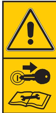
Shut off engine and remove key before performing maintenance or repair work
