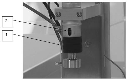
Pull the clutch casing sleeve (1) down, and turn the capping head until the hole in the adjustment lock plate is visible through the slot (2). Insert a Phillips Screwdriver and adjust torque by turning. Increase capping torque by turning clockwise.
