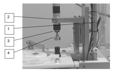
Loosen the finger screw (1), move the air motor (2) to the upper position and fasten the finger screw. At the same time pull down the spring-loaded release sleeve (3), and the capping head (4). The capping head will come off the quick change chuck.
