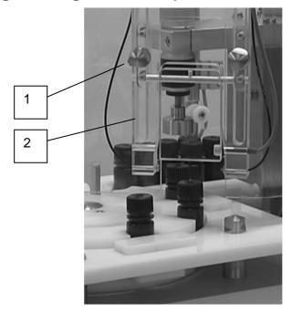
Loosen the finger screws (1), and lift up the gate (2). Place a bottle with a loosely screwed cap in the slot where the bottle enters the guarding. Close the guarding and lower the gate until the distance between the cap and the small gate is 2 - 4mm. The optical sensor will now detect the cap as it passes.
