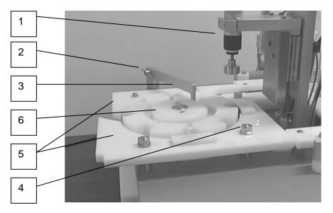
Elevate the capping machine (1) if necessary.
