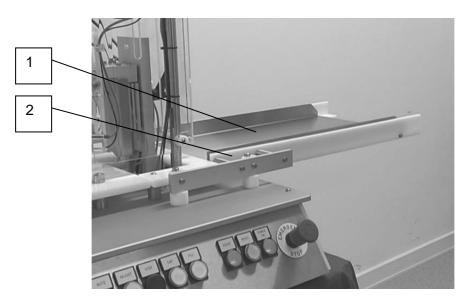
The collecting tray (or tray loading device) (1) is fitted to FF30-S screw capping module by the supplied screws (2) (4 pcs. M6x65).
