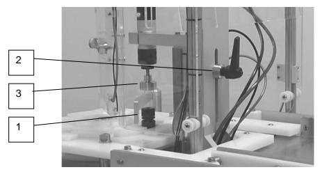
Place a bottle with fully screwed cap (1) in the capping station. Close the guarding and press RESET. Now press ADJUST, and the capping head will come down towards the bottle. While the machine is in adjust-mode, is it possible to open the rear guarding without having an alarm from the safety
