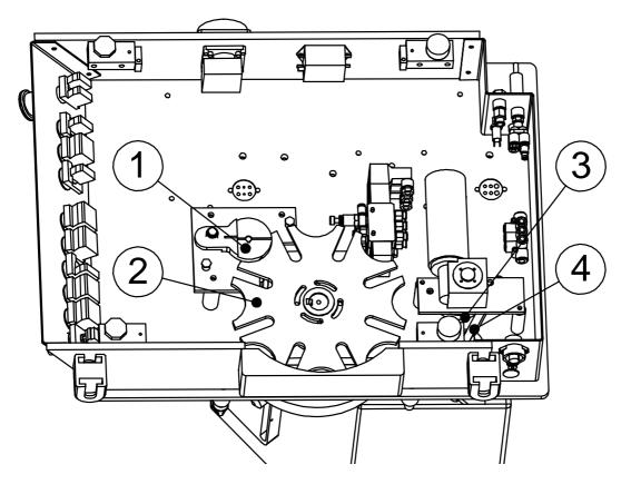
The contact faces between the cogwheel (1) and the Geneva wheel (2) should be lightly lubricated with a suitable grease such as Dow Corning MOLYKOTE grease BR2 Plus. The contact faces between the eccentric hub (3) and the ejector arm (4) should be lightly lubricated with a suitable grease such as Dow Corning MOLYKOTE grease PG75.
