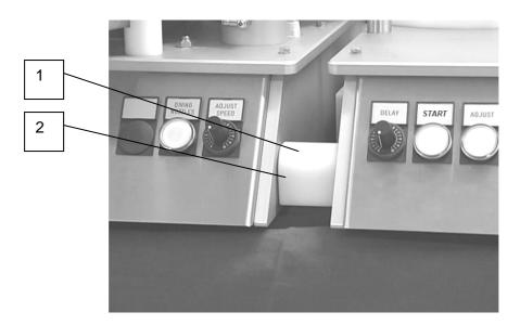
The FF30-S is connected to the feeding module by fitting the couplings (1) to the locks (2). This connection aligns the modules horizontally.
