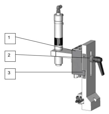
The height of the capping set can be set by the use of the scale on the side of the stand holding the screw capper.
