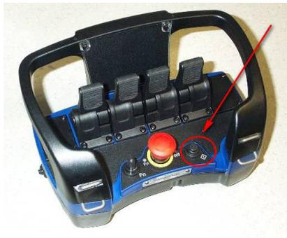
3) Press the switch on pushbutton on the PCU and keep pressed for about 4-5 seconds until you hear a short BEEP.
