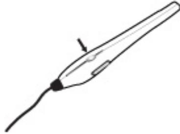
8. If you have purchased the optional Foot Switch, you can use it in place of the Capture button on the camera. When the Foot Switch is plugged in and one of the two foot pedals is pressed, the Capture button on the camera will be disabled until the Foot Switch is removed and is no longer detected. The blue C pedal is used exactly like the Capture button on the camera. The red M pedal toggles between live video and previously stored images.
