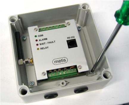
1. Loosen the fixing screws (4pcs) and take the module out from the enclosure.
