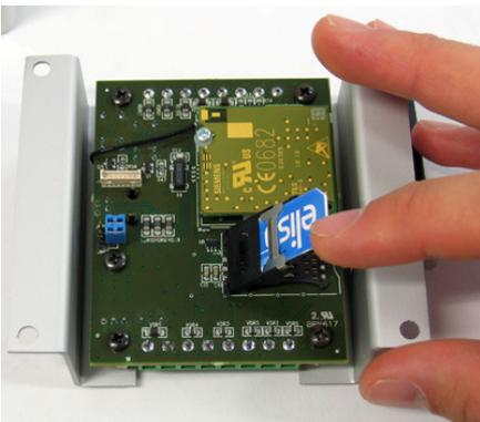
3. Install the SIM-card so that the sloped footing is outwards like in the picture.
