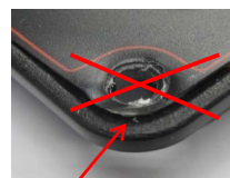
Over Tightening Causes Failures
