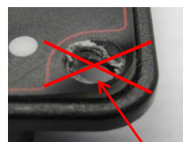
Over Tightening Causes Failures
