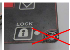
Lock Washer Damage
