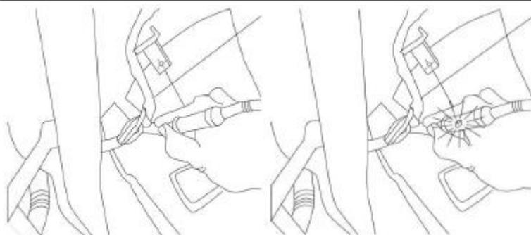
**The high-level detection mechanism is:** When the vehicle door is closed, the voltage of door pin switch is low-level. When the vehicle door is open, the voltage of door pin switch turns into high-level, and the main unit judges that the door is opened;
