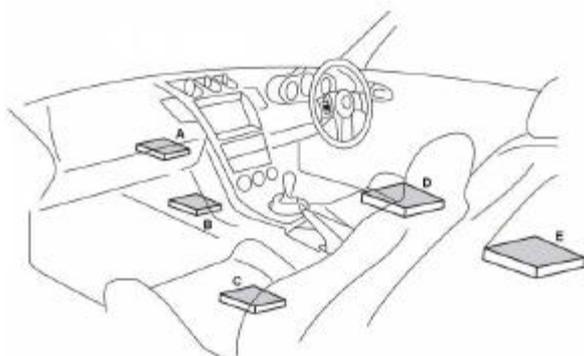
Magic tape can be used to fix the main unit to the vehicle body.
