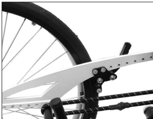
The brake mechanism is attached by two screws.
