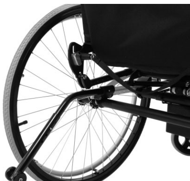
Anti-tip protection in down position.
