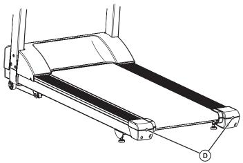
If the striding belt moves to the left, turn the left tension bolt a quarter-turn clockwise and then turn the right tension bolt a quarter-turn counter-clockwise to start striding belt tracking back to the center of the roller.
