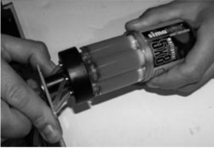
Remove protection cap. Snap simalube multipoint onto the connecting adapter. Pay attention that the lubricator is correctly attached.
