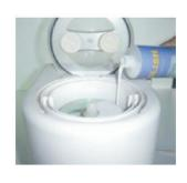
Set the timer on 5 minutes. The repair process starts.
