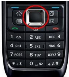
Figure 2. On this phone model, the navigation key (circled in red) doubles as the arrow keys.
