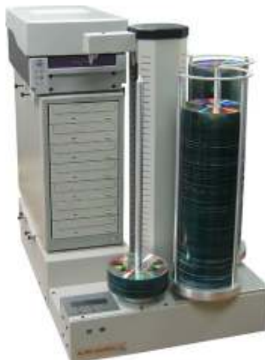
Fig. 4c System configured with 7 drives and Rimage printer
