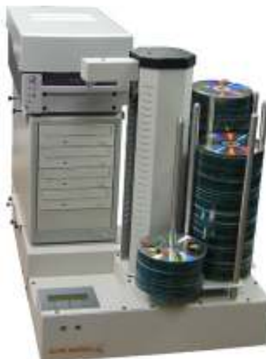
Fig. 4a System configured with 4 drives and Rimage Prism Plus printer
