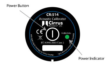
The calibrator will automatically switch off after 5 minutes to preserve battery power.
