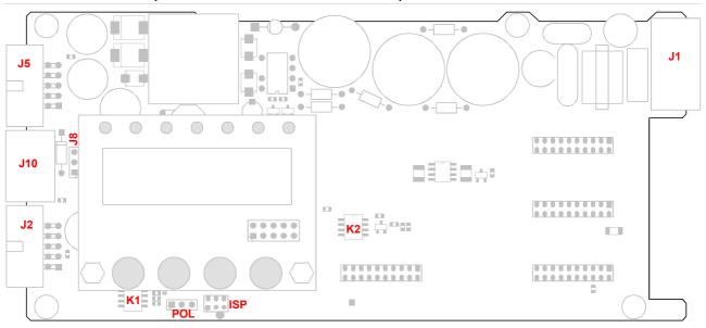
The DIP switch positions, read from top downwards. K2.2 means the second switch of K2.
