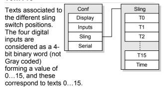
T0 is displayed when all the digital inputs are non-active. T1 is displayed when the lowest input is active (terminal C4), T2 when the second lowest is active, etc.
