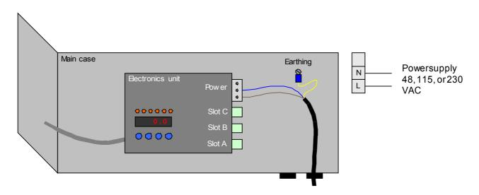
Bring the Live and Neutral wires to the electronics unit as in picture. A pre-fuse is not necessary, but if one is used, it should be at least 1 AT.
