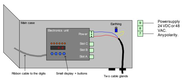
Bring the supply voltage to the connector indicated in the picture. It is recommended to earth the enclosure using the M4 screw provided for additional protection against disturbances. A pre-fuse is not necessary, but if one is used, it should be at least 2 AT.
