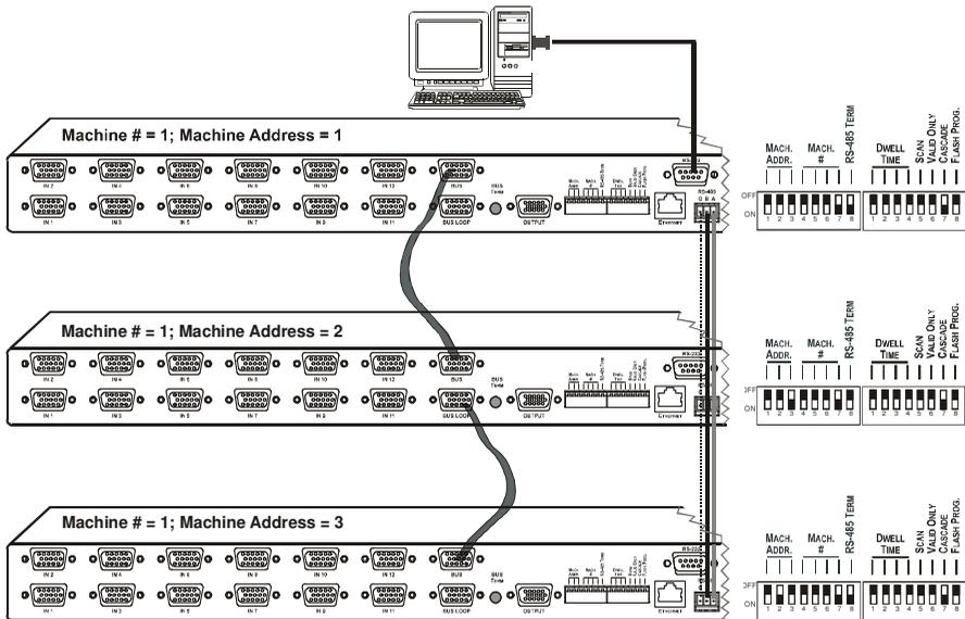
Figure 26: Connecting VP-1201 Machines – Input Expansion Configuration
