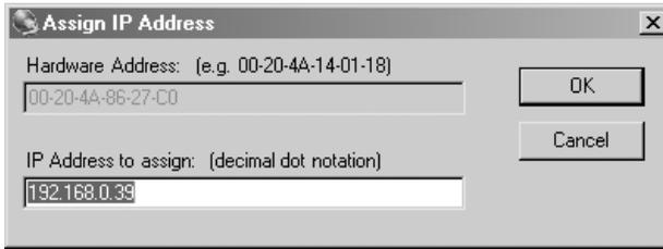
Figure 10: IP Address Assignment Dialog Box
