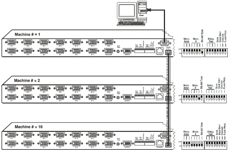
*Figure 25: Connecting VP-1201 Machines – Individual Control Configuration*
