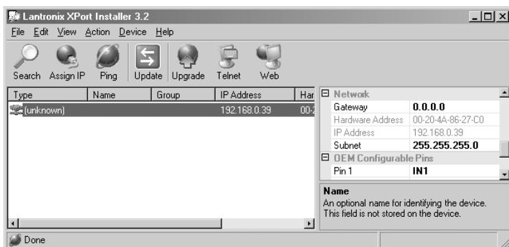
Figure 9: Device Found on the Network
