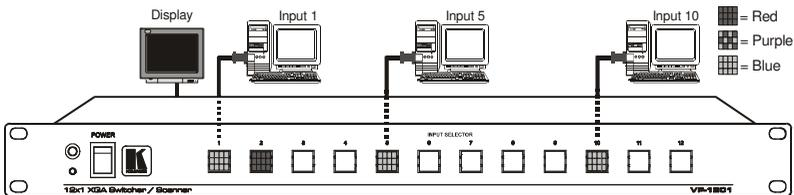
Figure 28: VP-1201 Input Buttons Illuminated (I)
