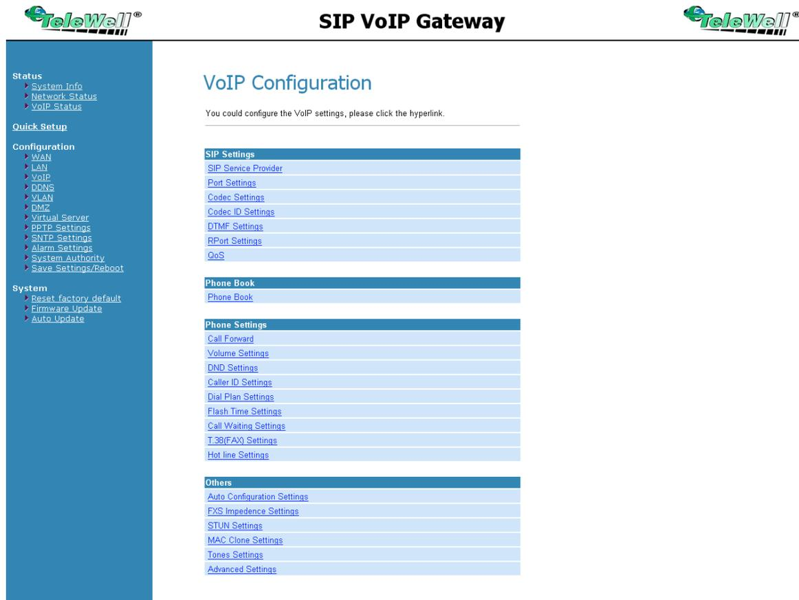
The screenshot displays the web interface for a SIP VoIP Gateway. The page title is "SIP VoIP Gateway" and the main heading is "VoIP Configuration". A message states: "You could configure the VoIP settings, please click the hyperlink." Below this message are several sections of configuration options, each with a list of hyperlinks:
