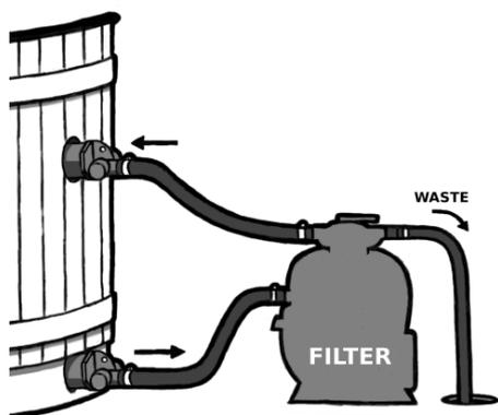
For the winter, or when the filter is taken out of service otherwise, the return hole must be closed with the supplied cover.
