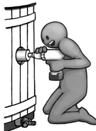
The Lead-in is connected to the plastic so that the rabbet of the sealing is on both sides of the barrel plastic and tightened securely.
