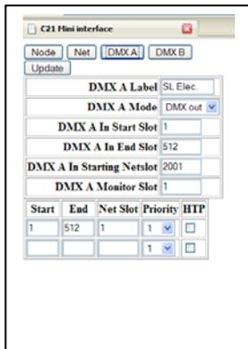
**DMX A Label:** This field contains a character string of up to eight (8) characters used to identify the function of the DMX Port.
