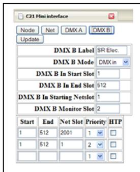
**DMX B Label:** This field contains a character string of up to eight (8) characters used to identify the function of the DMX Port.
