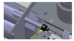
Hold the flame sensor's rubber cap and pull the flame sensor carefully from its pipe.
