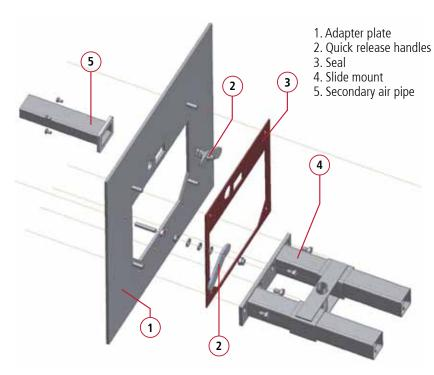
Mount the quick-release handles, slide mount and secondary air pipe as shown in the photograph.
