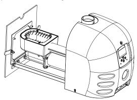
Mark out the points for the boiler's mounting pins, and drill holes at the marked points. The seal between the adapter plate and the boiler should be made with sealing tape or equivalent.
