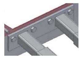
Install the slide mount according to the figure. The final attachment of the slide mount is done when the burner is attached to the adapter plate. The slide mount is lifted up against the slide mount fastening pin and the screws are tightened.
