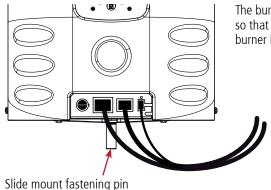
The burner cables should be attached to the boiler so that the plugs must be removed from the burner before it is pulled out of the boiler.
