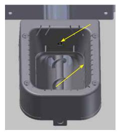
Clean the burner bowl of ash and any sintering. The primary air ring's air holes and the firing element's holes should be open.
