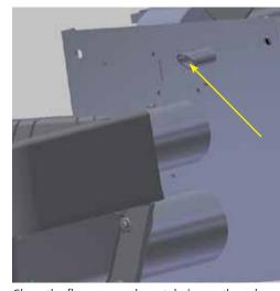
Clean the flame sensor's metal pipe so the ash that has collected in the pipe does not prevent the flame sensor from working.
