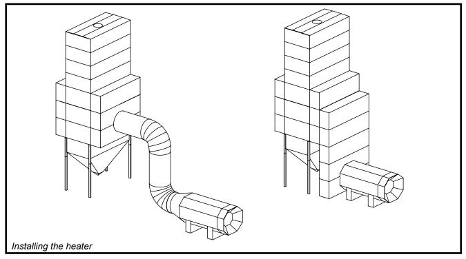
The debris pipe from the pre-cleaner must be equipped with a cyclone or equivalent for separation of debris. The separator must be located on the same side with the outlet air duct or entering of dust or debris into the suction opening of the heater must be prevented by some other means.
