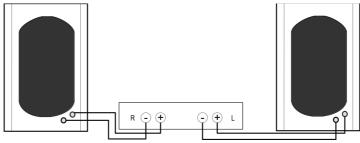
On the back of Gradient 5.0 attach the positive lead to the red connector and the negative lead to black connector.
