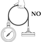
cannot be bended under a radius of 150mm and it is recommended to fit it so that it is not subject to vibrations. The difference in height between the instrument and the diaphragm seal causes an hydrostatic effect on the measuring instrument and subsequently a variation in the instrument indication range. If known, this difference value must be indicated in the order otherwise the instrument must be reset on site.
