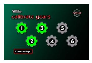
This page requires configuration while the vehicle is in operation and, therefore, requires an assistant. The vehicle must be in operation (i.e., driving on a quiet safe road where each gear can be selected and held for a few seconds).
