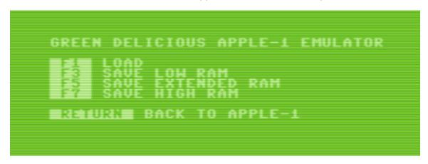
Low RAM is \$0000-\$0FFF (4K), Extended RAM is \$0000-\$3FFF (16K) and High RAM is \$6000-\$EFFF (4K).
